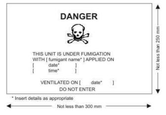
**3.15.4.** Recommendations on the Safe Use of Pesticides on Ships Contains a warning sign for fumigated vessels, ship compartments, cargo containers, and fuel vessels. The IMO / ILO / UN ECE Guidelines for the Packaging of Freight Transport Units (CTUs) are included.
